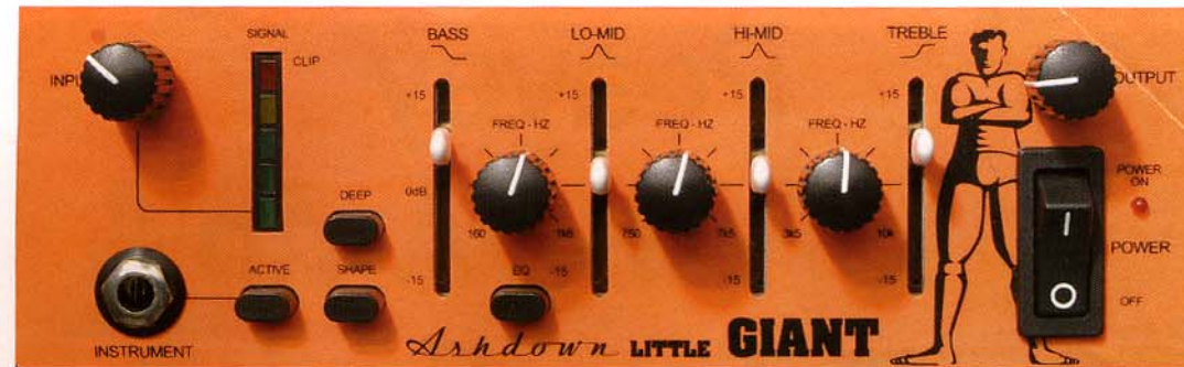
Preamp has presets, semi-parametric, and shelving EQ options.
